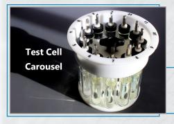
The BLB Test Cell Carousel accommodates twelve (12) samples, allows convenient alignment of each cell to the appropriate test position, and holds both  $\mathsf{SimAir}^{\mathsf{T}}$  and DIN glassware.
